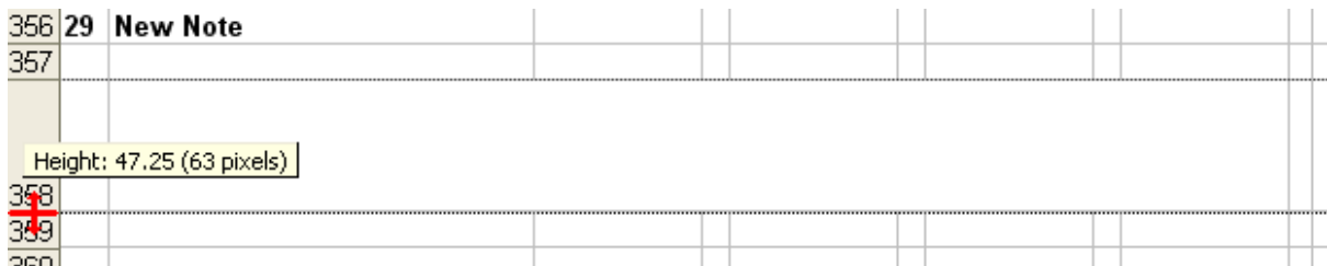
Screenshot showing how the cursor changes into a cross when held over the line between the row numbers (the cursor is actually in black; red has been used here to make it more visible)
